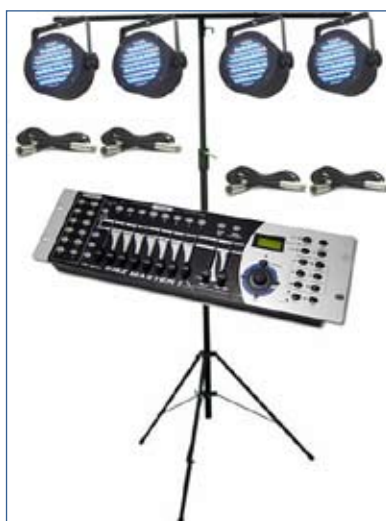
Figure 7. DMX Lighting system
